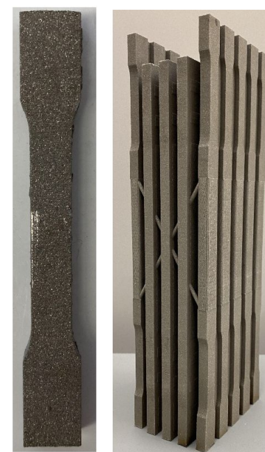
Figure 1.1: Real, titanium alloy additive manufactured test coupon
